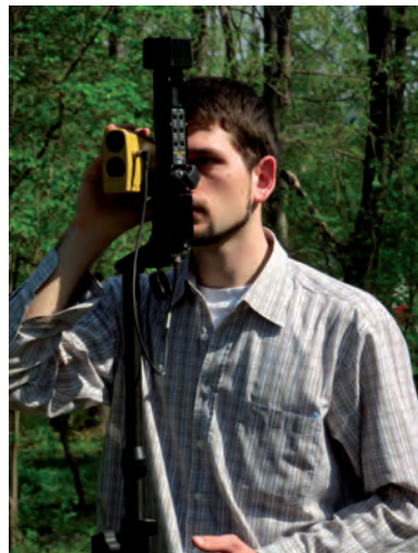
3. ábra: A terepi mérés TruPulse-zal és MapStar Compass Module II-vel. Figure 3: Surveying with TruPulse and MapStar Compass Module II.
